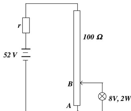
If the distance from A to B is 5 cm, what is the internal resistance,  $r$ , of the supply?
